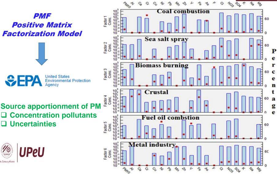
Atmospheric aerosol or particulate matter – possible emission sources
